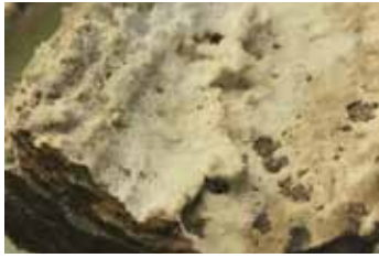
Figure 2. Cross-Section of carbonaceous scale build up.
