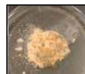
Figure 3: Calcium Carbonate scale removed from scrubbers
