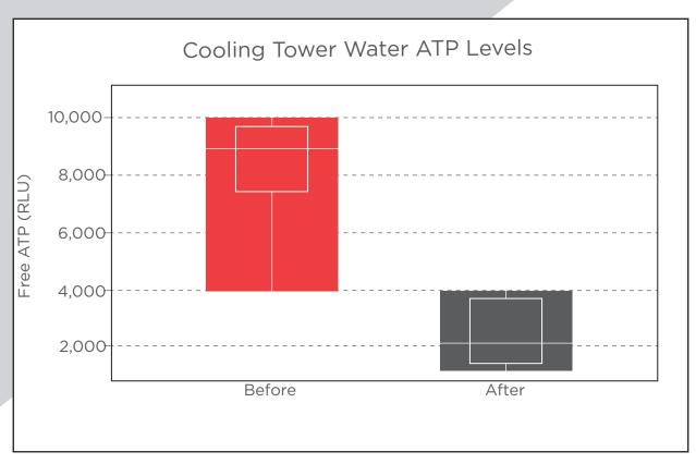
(Above) Before Hydrite's EPA registered peracetic acid addition, slime forming bacteria levels were high resulting in poor heat transfer and frequent cooling tower packing (fill) replacements. After Hydrite's peracetic acid addition, cooling tower slime forming bacteria was dramatically reduced and cooling tower performance increased.
