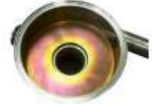
This is an example of rouging stain which is a corrosion product.
