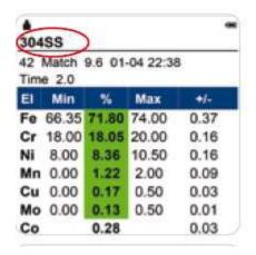
In the pictures below, you will see a valve body with a discolored section. Using the Bruker XRF Analyzer, we were able to show the customer that the discolored section of the valve had a slightly inferior chemical composition.
